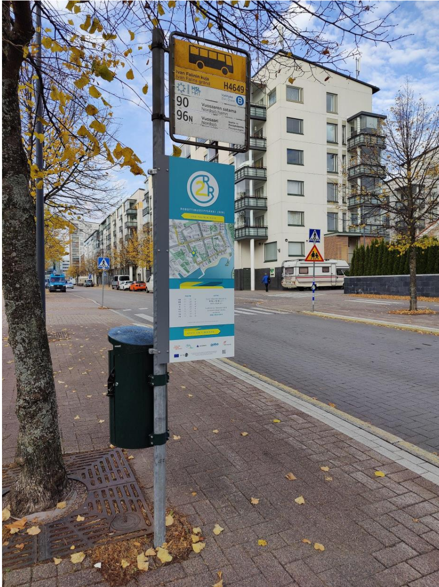
Figure 12: Ride2Rail robobus bus stop sign mounted on regular HSL bus stop pole [Rutanen 2021]
